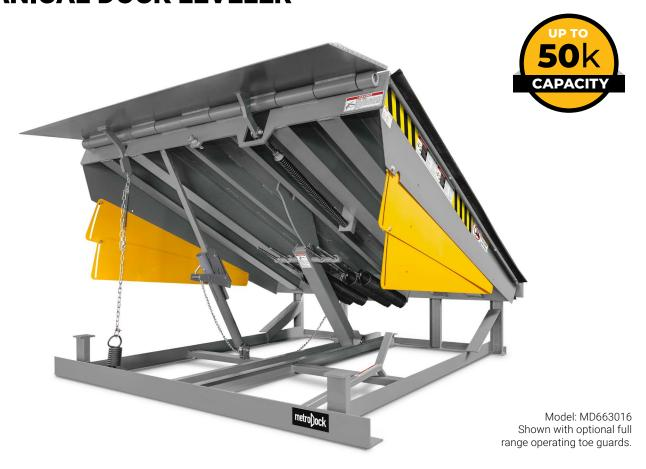
The Mechanical Dock Leveler is manually operated and easy to use: to operate, simply pull the release chain located at the rear of the deck; the dock will rise and the lip will extend; at which point the dock leveler can be walked down onto the truck bed for safe loading or unloading.
