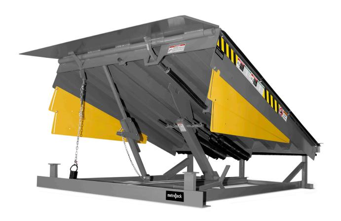
The mechanical leveler is manually operated and easy to use: to operate, simply pull the release chain located at the rear of the deck; the dock will rise and the lip will extend; at which point the dock leveler can be walked down onto the truck bed for safe loading or unloading.
