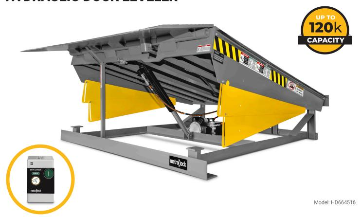
**Hydraulic Dock Levelers:** Simple to use, durable, and cost-effective, with a standard capacity of 30,000 lb. and optional capacities up to 120,000 lb. They feature single push-button operation, constant pressure for added safety, and rear hinge tilt to handle uneven truck load approaches. Built with premium North American components, Metro Dock hydraulic dock levelers come in formed beam or I-beam designs, with 1HP power packs available in any voltage.
